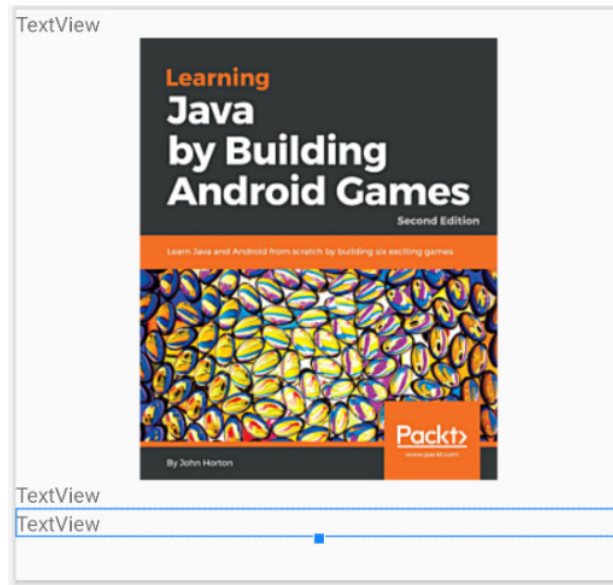
Figure 5.8 – Making the layout look nicer by adding sp, dp, and gravity attributes
