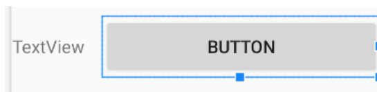
Figure 4.13 – Dragging a Button widget from the Button category onto the right-hand side of the previous TextView widget
