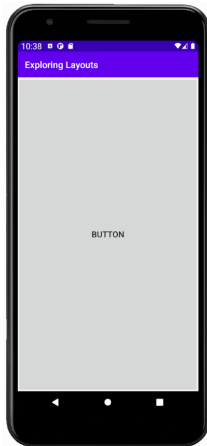
Figure 5.2 – The button expanded in both height and width to match the parent
